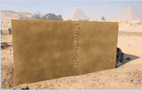
Left: A mudbrick test wall segment shortly after it was erected in 2005 to test the effects of weathering and erosion over time.
