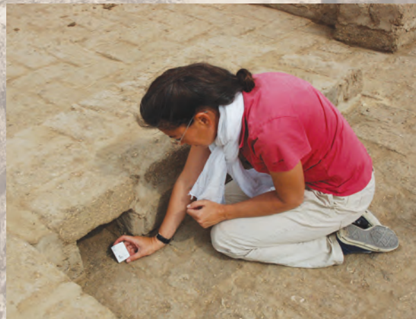
Step 4: We installed two small monitors above the ancient walls to record humidity and temperature variations over a period of one year. Ana Tavares, director of the conservation project, positions the monitors.
