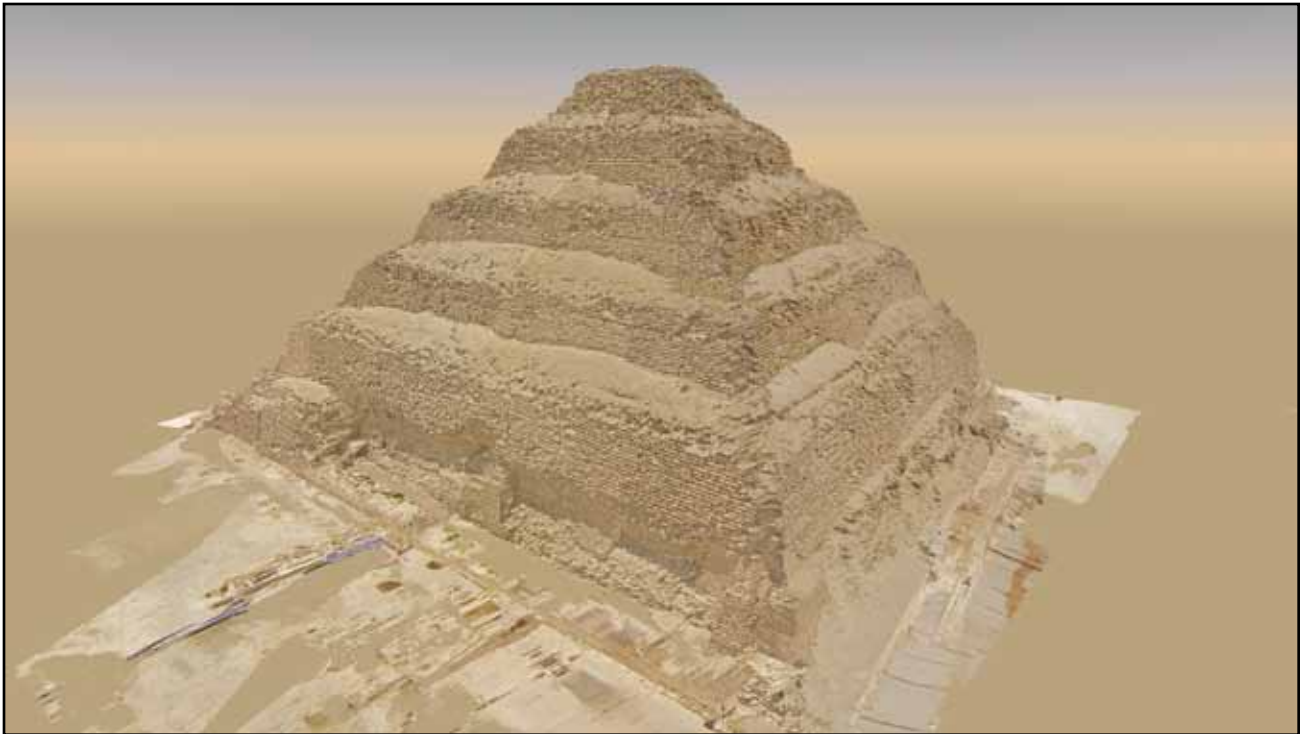
Plate 7.1. Preliminary version of the point cloud model of the Djoser Step Pyramid produced by GLS-1000. View of the southwest corner, looking northeast. Gaps remain until data from the Zoser Scanner are fully incorporated.
