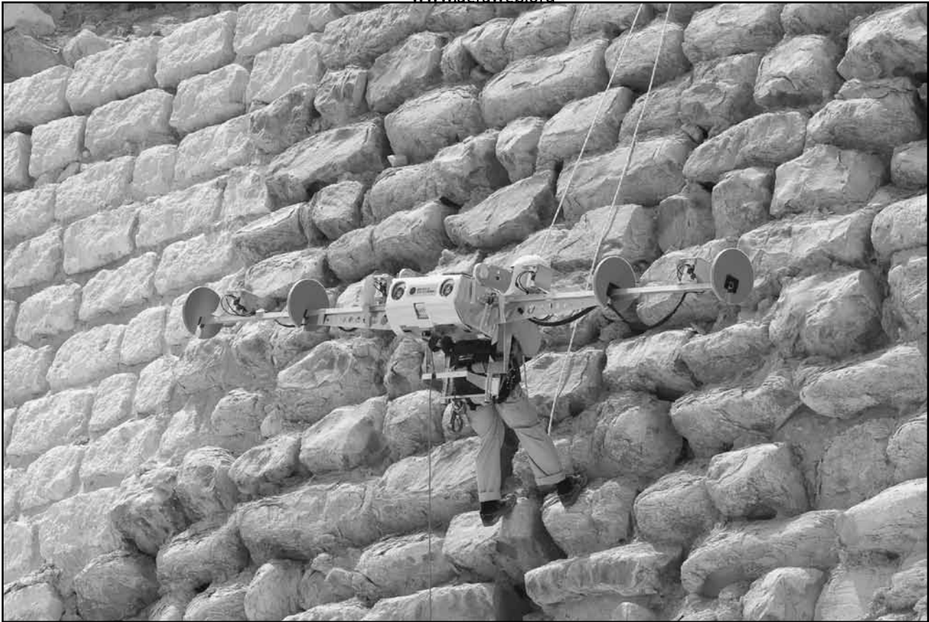
Figure 58. Yamamoto carries the Zoser Scanner on his back as he rappels down a face of the Step Pyramid. The Zoser Scanner laser-scans and photographs during the descent. Rappelling down the southern side. Photo by Yukinori Kawae.
