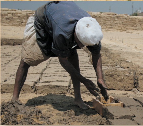
A brickmaker forms mudbricks in a wooden mold, lining them up along the ground to dry. Up slope, piles of Nile sediments and bags of straw are ready to be mixed for bricks in a mixing pit far in the background. Photo on left by Hilary McDonald, large photo by Ashraf Abd el-Aziz.
