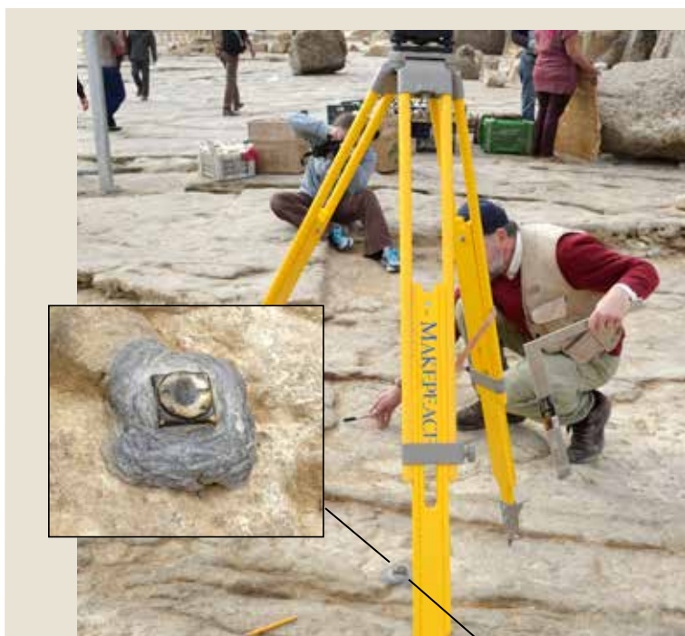
On the south side of the Great Pyramid there was no direct evidence of where the casing stones met the platform. In order to project where the casing stones once would have fallen on the platform below, Glen Dash measures the top outer edge of the casing stones, assisted by Rebecca Dash. Photo by Mark Lehner.
