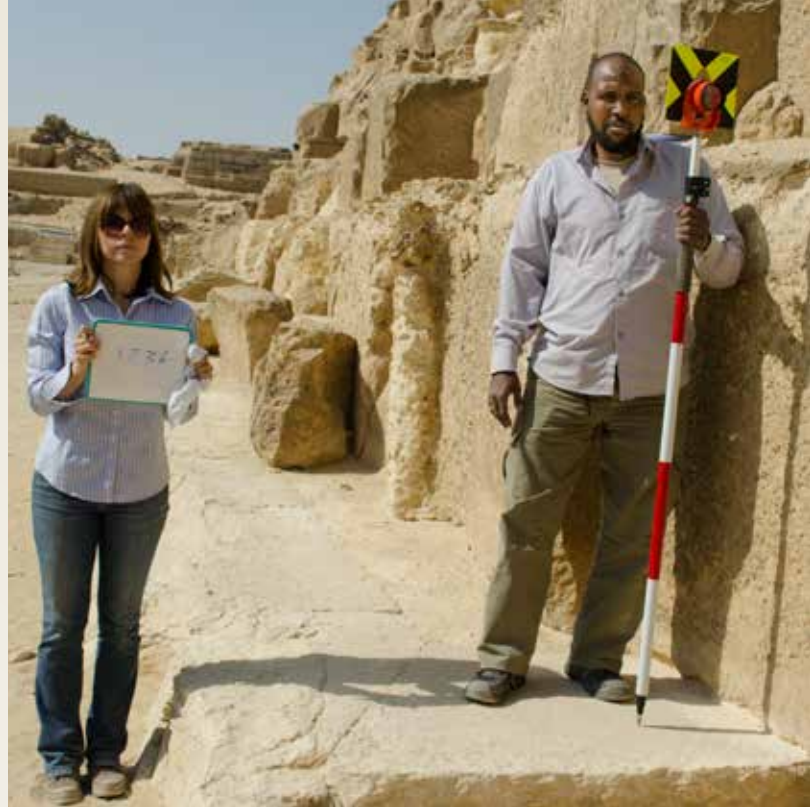
For a photographic record of each point we surveyed, Joan Dash holds a board with the point number, while Mohammed Abd el-Basset, surveyor with Egyptian Ministry of Antiquities, holds a rod with a reflector mounted on its top over the point. This point is on the pyramid's platform on the south side just to the west of the surviving casing stones. Photo by Ashraf Abd el-Aziz.
