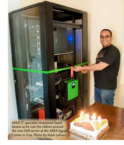
The Dell server can also be counted on for reliability and security. Its backup power source can provide 1500 watts to keep the machine running for up to two hours during power outages. A backup server assures that all files are protected from loss. And as the Dell supports the latest security technology, cyber threats are kept at bay. In addition, the server alerts the administrator to hardware failures, and with its fail-safe support, it will continue working even with damaged hardware.
