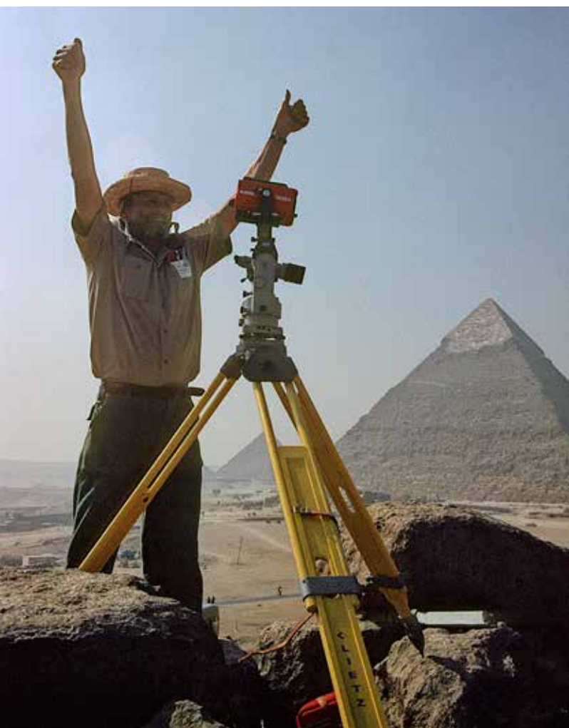
David Goodman, "at the gun," signals that he has taken the angle measurement with the theodolite, and the distance measurement, with the Red 2A EDM, so the target reflector and tripod can be removed from survey point GP11, atop queen's pyramid GI-c, during the 1984 season.
