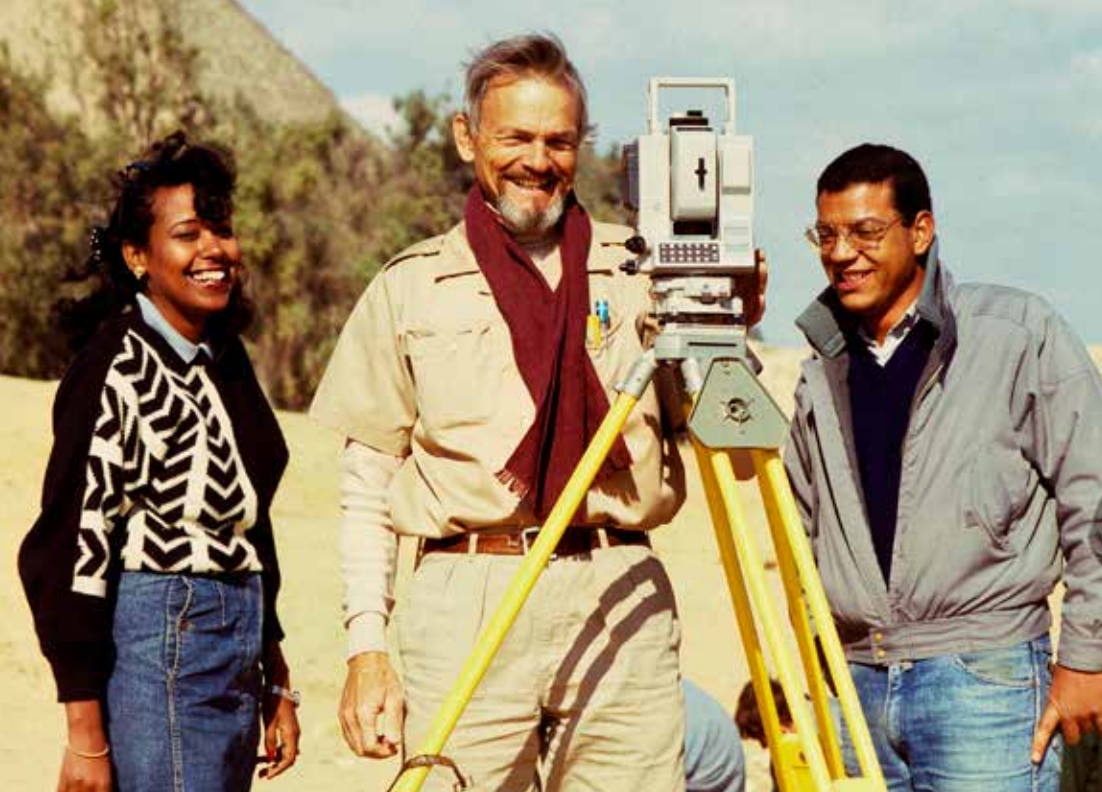
David Goodman surveying during season 1988, now with a Total Station (theodolite and electronic distance measurer combined), while teaching use of the Total Station to Inspectors Nemat Hamed Mohamed (left) and Maher Moussa (right).
