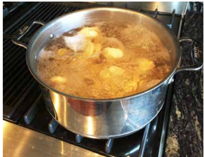
Boiling the distal and proximal ends of the limb bones of a sheep to test in the drop tower.
