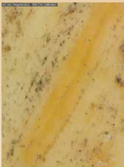
B. Metal cut mark, 220× magnification
