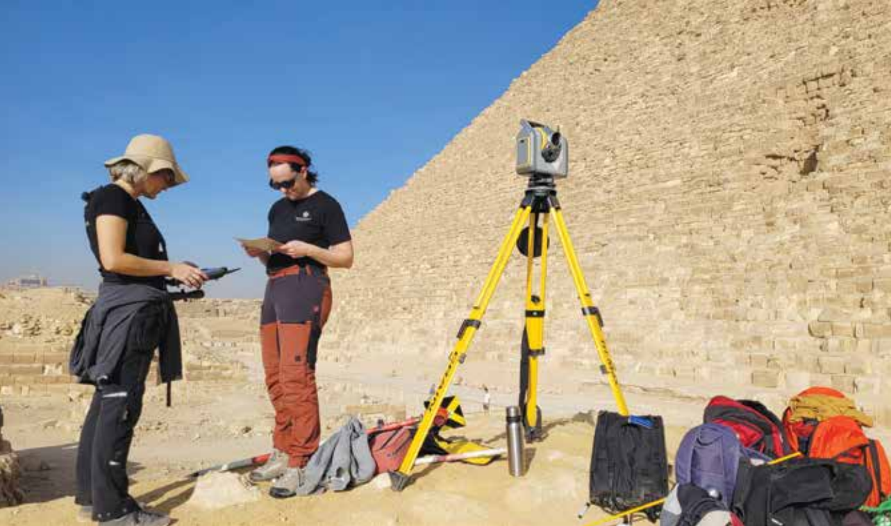
Sarah Skytte Qvistgaard and Dr. Sarah Croix set up the laser scanner at the Great Pyramid. The Trimble SX10 scanning total station combines automated total station positioning with band scanning using a rotating prism telescope. Photo by S. Saleh Abd el-Hakim.
